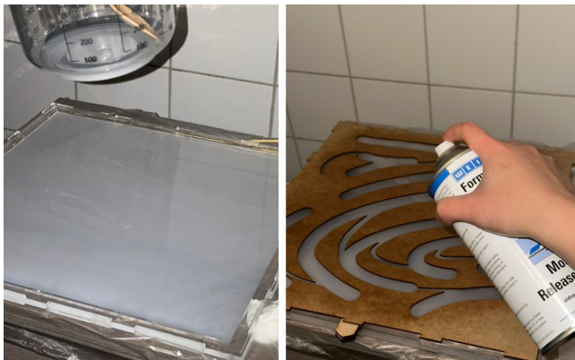
Figure 7 Silicone layer fabrication process
