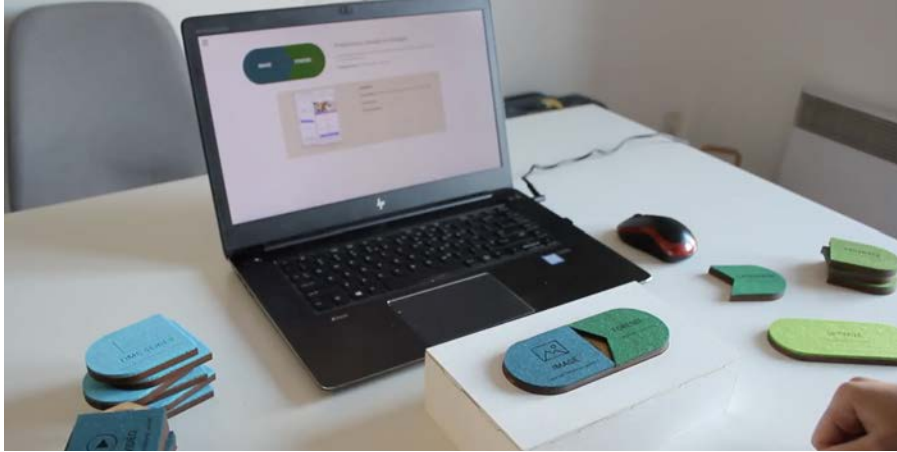
Fig. 1: The original version of the toolkit with the sensing board, sensorized tokens and web interface
